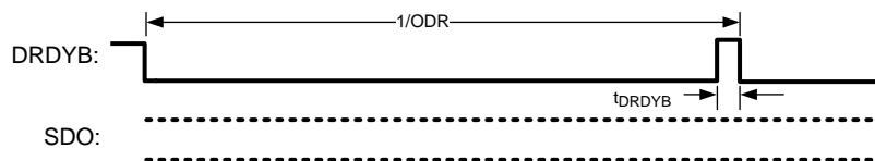
Figure 21. DRDYB Behavior for an ADC_DOUT not Read
