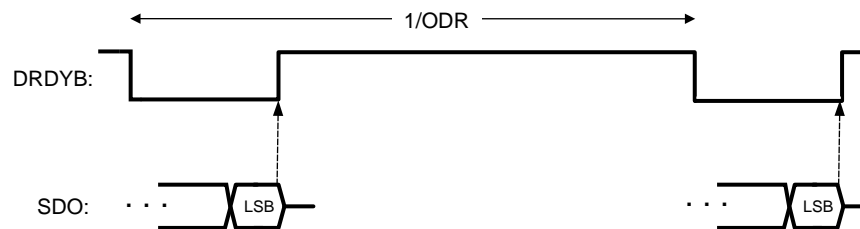
Figure 20. DRDYB Behavior for a Complete ADC_DOUT Reading
