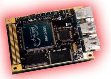
The DAI3 Module from ZP Engineering in conjunction with the eBebob I/O Board offers the full range of Bebob 5.x options, for both 1394- and USB2.0-based applications.
